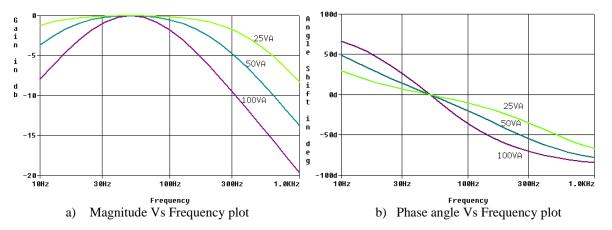
Fig.7. CVT frequency response with variation of burden magnitude
