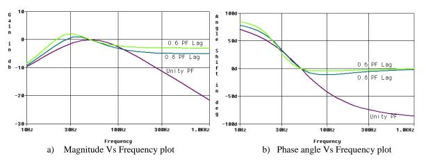
Fig.6. CVT frequency response with variation of burden power factor
