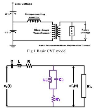
Fig.2. Equivalent circuit of CVT
