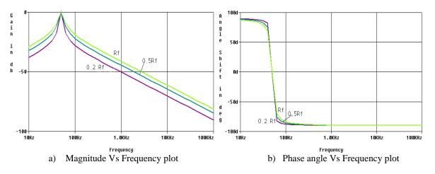
Fig.4. CVT frequency response with variation of Ferroresonance suppression resistance
