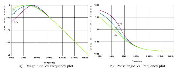
Fig.5. CVT frequency response with varaiton of capacitance
