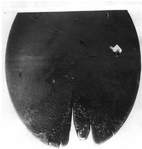
Fig. 7 Fractured plate of Valve No. 3 Source: Z.W. Yu and X.L. Xu (2006) [8]
