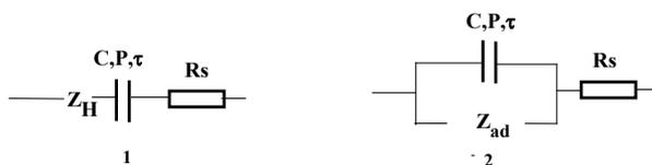
**Figure 3.** Equivalent circuit models for stainless steel in 0.10 M  $K_2SO_4$ .
