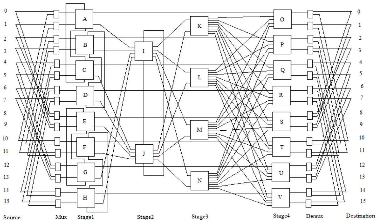
Fig. 4. Irregular Modified Shuffle Network (IMSN)
