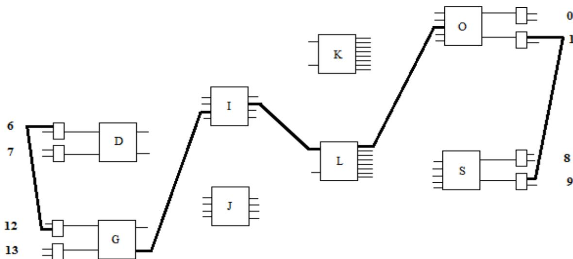
Fig. 7. Routing of data packets from source 6 to destination 9 in faulty case
