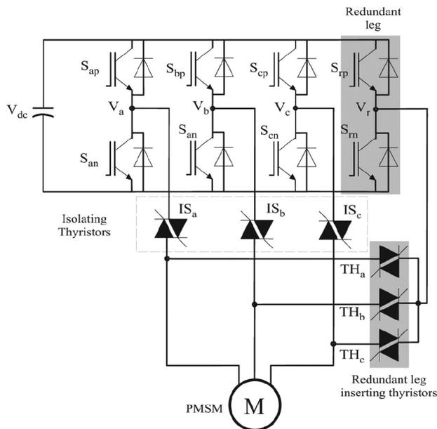
Operation for the single IGBT open circuit fault:
