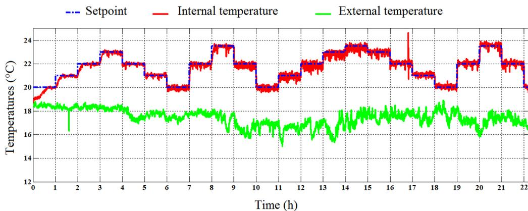
Fig. 9 Variations of external, internal and set-point temperatures.
