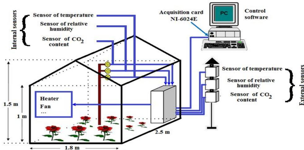
Fig. 1 Schematic view of the greenhouse system.
