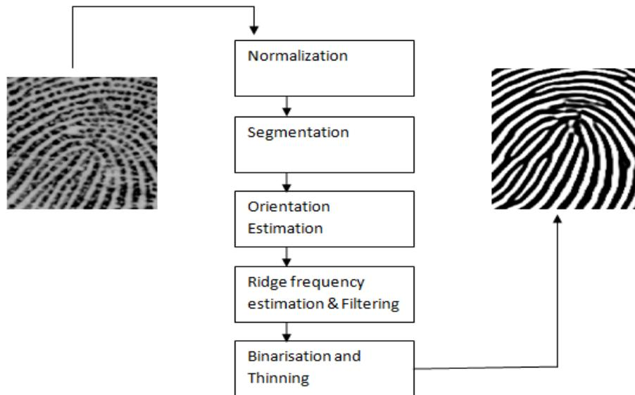
Fig 3.2 flow diagram of fingerprint enhancement
