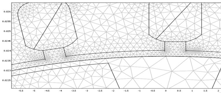
Fig 2: Meshed Plot at the air gap
