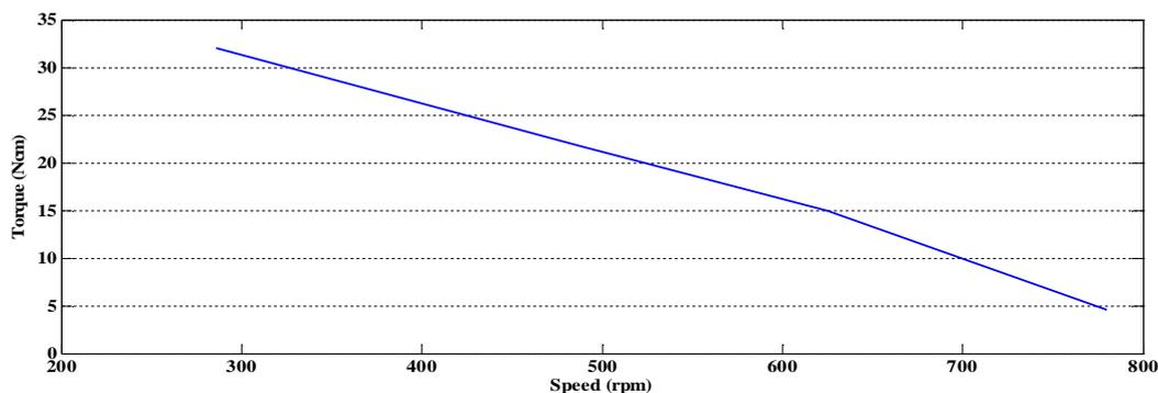
Fig 13: Torque-Speed Plot
