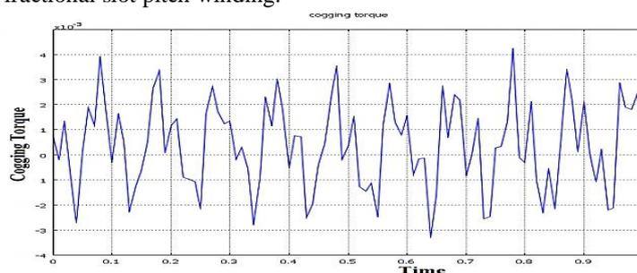
Fig.7: Cogging Torque
