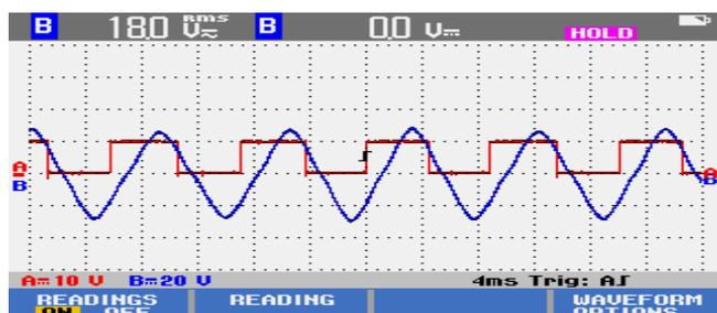
Fig.11: Hall sensor signal and back EMF waveform
