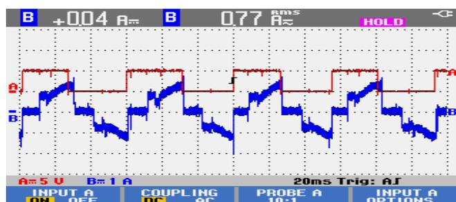
Fig12: Current wave form of phase A during clockwise rotation.
