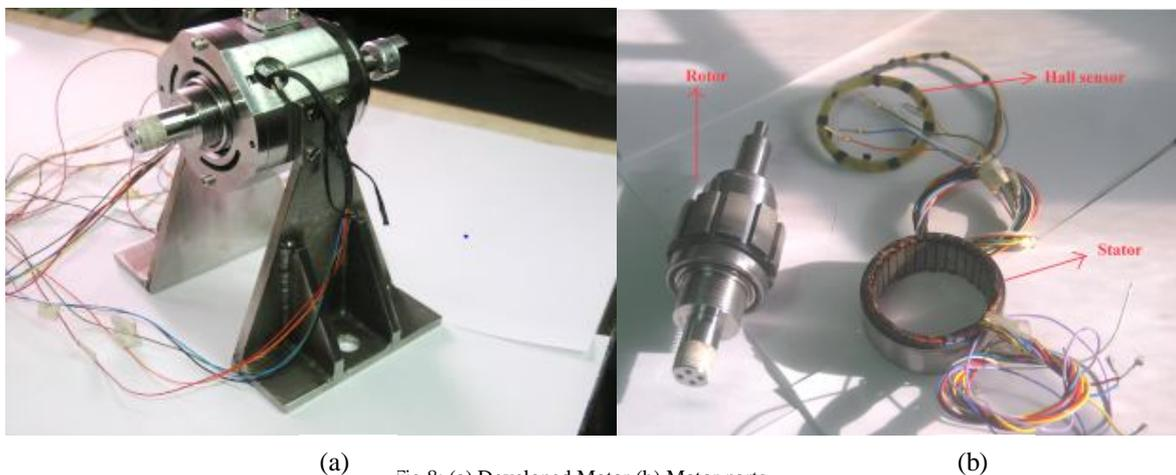
(a) Fig.8: (a) Developed Motor (b) Motor parts
