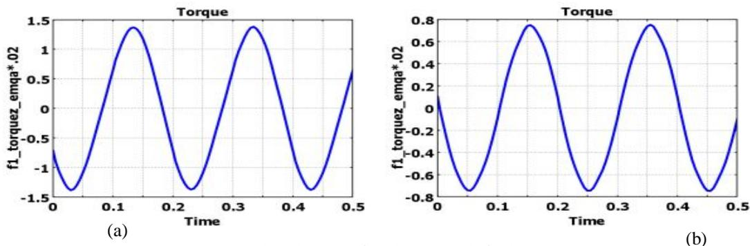
fig 4: Torque Vs time plot (a) For five phase motor (b) for three phase motor
