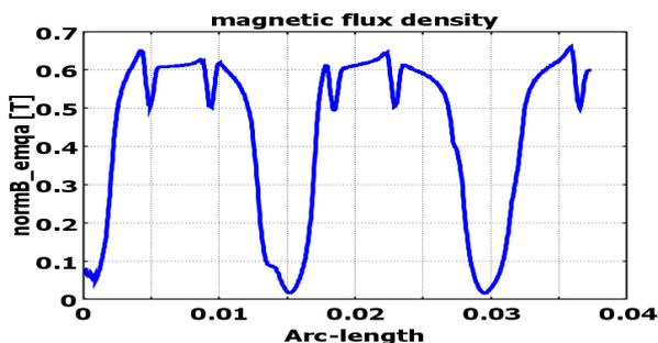
Fig.5: Magnetic flux density at the air gap
