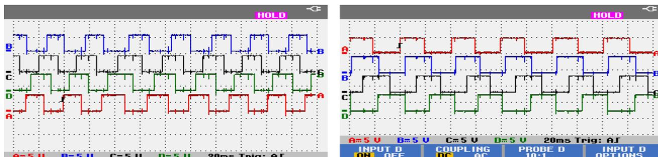
Fig.10: Hall sensor Signals for 4 phases (a) Clock wise direction (b) Anti clock wise direction
