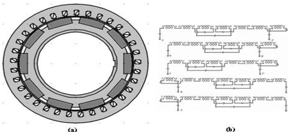
Fig 1. (a) Designed motor model with permanent magnets (b) Winding diagram
