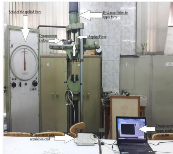
Fig. 4. Dynamometer calibration set up.
