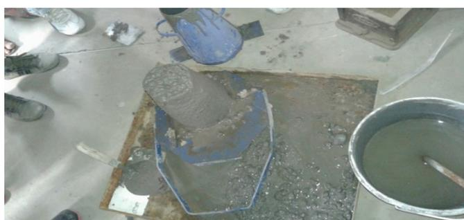
**Figure 8.** Slump test.
