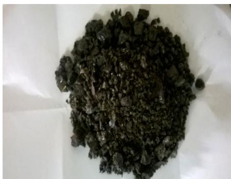
**Figure 2.** Basic oxygen furnace slag.
