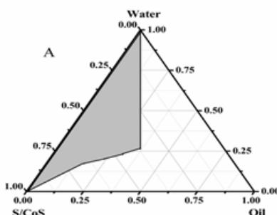
**Figure 1.** Pseudo ternary phase diagram composed of BJO and Capryol 90 (1:1, w/w) as oil phase, Labrasol and Cremophor RH40 mixed at the ratio of 1:3 (w/w).
