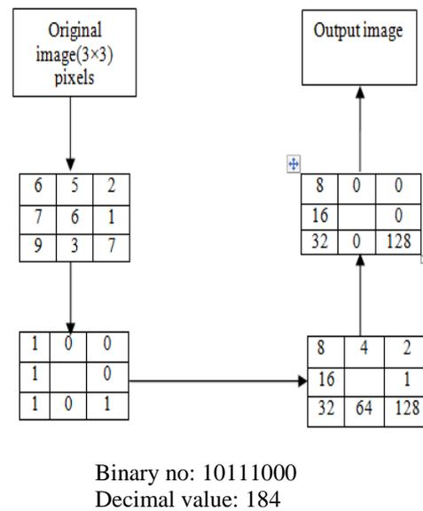
Fig.1. Example of local binary pattern operator
