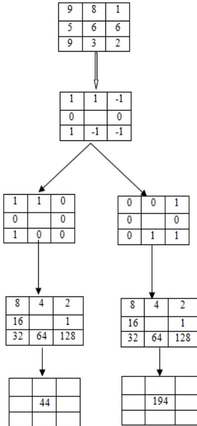
Fig.2. Calculation of LTP operator
