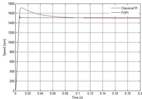
Fig. 11 Speed Response Comparison between Classical PI & FOPI
