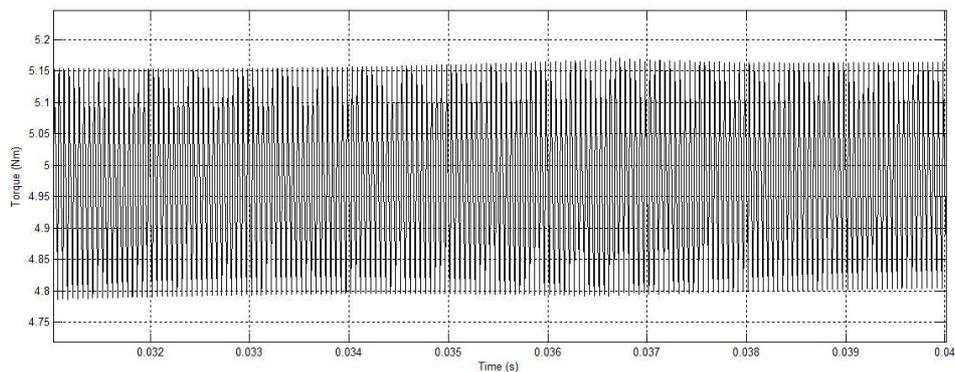
Fig. 12 Torque response of Vector Control of PMSM Drive
