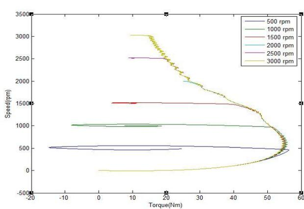
Fig. 5 T-N Characteristics of Proposed Drive.
