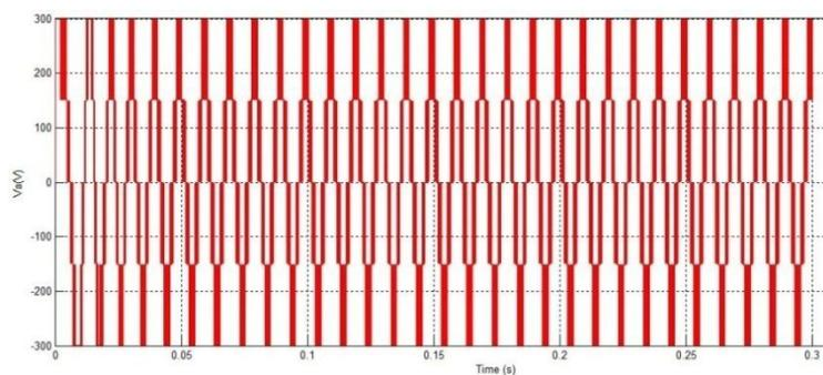
Fig. 4 Inverter Output Voltage.
