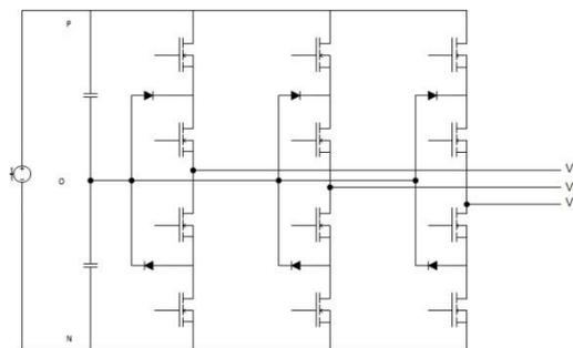
Fig. 1 Three Level Inverter Model
