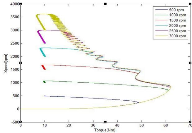
Fig. 6 T-N Characteristics of FOC of PMSM Drive.
