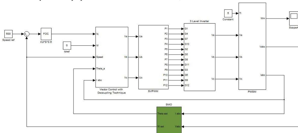
Fig. 3 Overall Simulation Diagram
