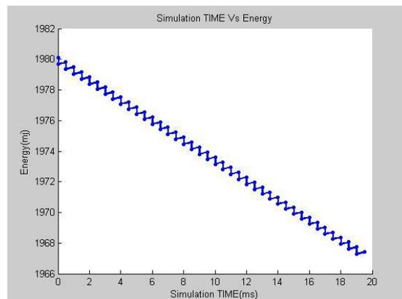
**Figure 7.** Energy with time in throughput maximization with energy restriction scheduler.
