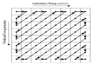
Figure.4. Raster scan order of dct coefficients
