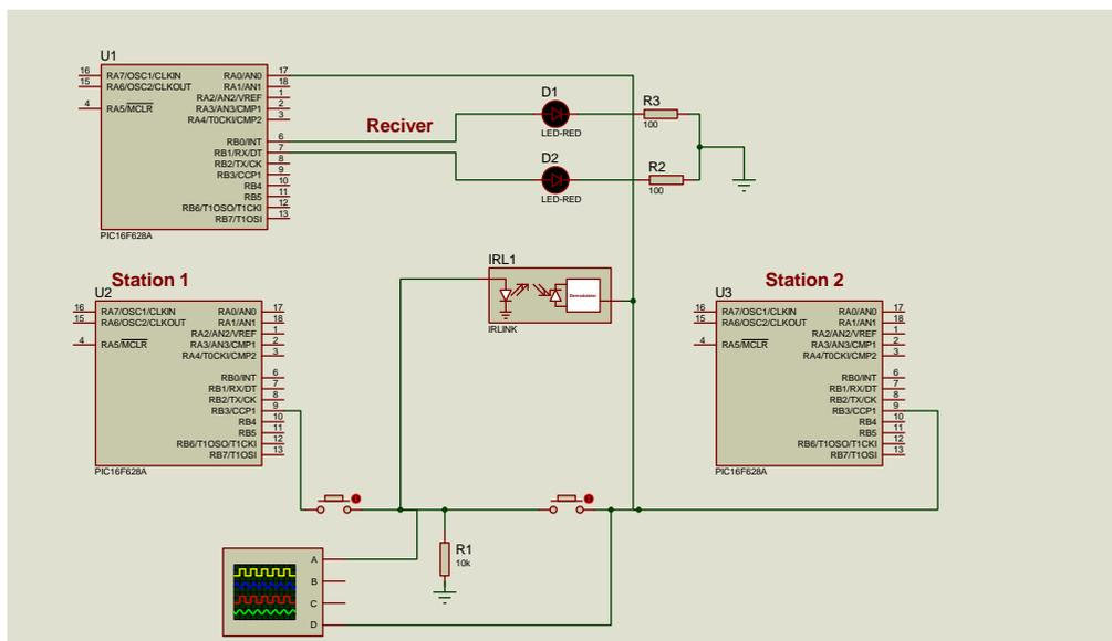
Fig 5. Schematic diagram showing the simulation of the IR sensors
