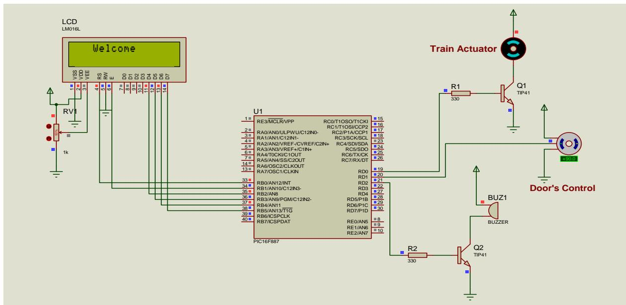
Fig 2. Schematic diagram showing the system simulation using Proteus software.
