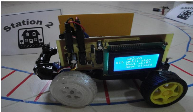
Fig 6. The assembled driverless train prototype
