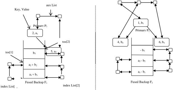
Fig.2.1: Two Fused Backups for toleratingtwo crash faults (Binary Search Tree)
