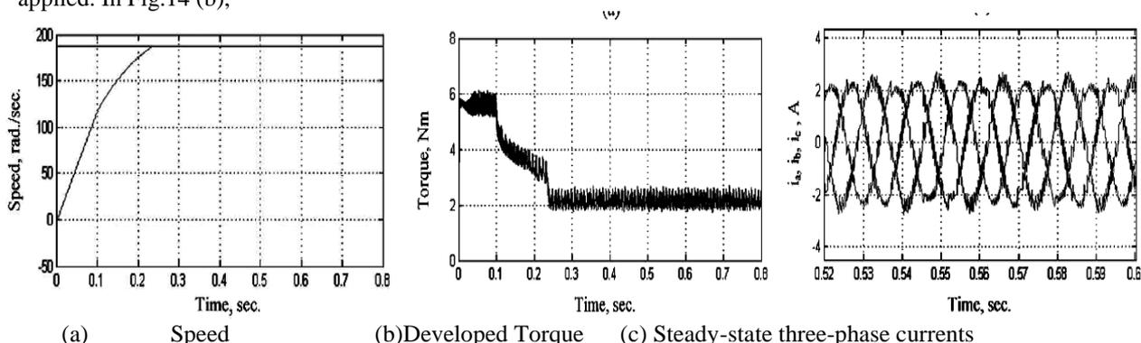
Fig.10. Simulation starting responses of the proposed Fuzzy based CSI fed Synchronous Motor (CSIFSM) drive at rated speed and rated load conditions.
