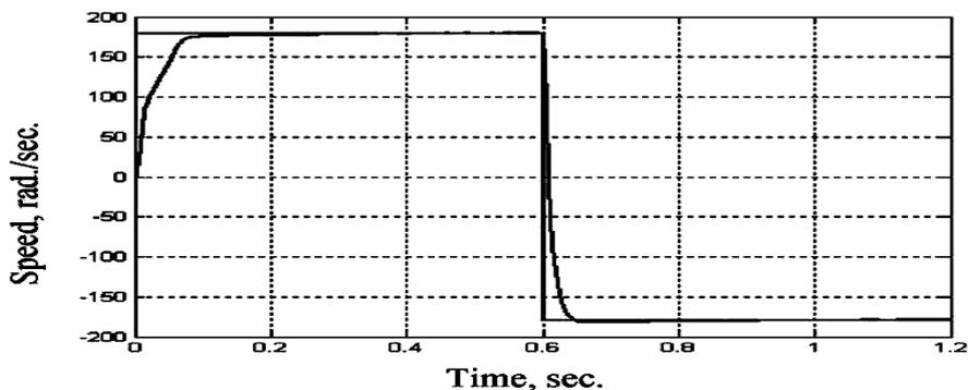
Fig.12. Simulated speed response of the proposed fuzzy based CSI fed Synchronous Motor (CSIFSM) drive for speed reversal of command speed.
