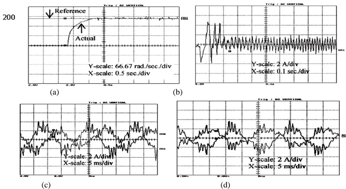
Fig.13. Experimental starting responses of the proposed fuzzy based CSI fed Synchronous Motor (CSIFSM). (a) Speed. (b) Stator current  $i_a$ . (c) Steady-state currents  $i_a$  and  $i_b$ . (d) Steady-state currents  $i_a$  and  $i_c$ .
