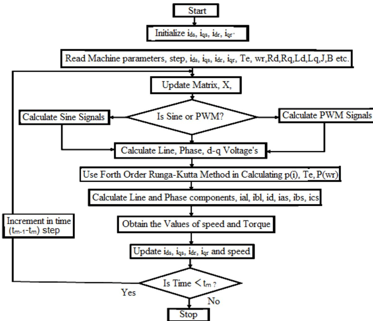
Fig.9 Flow charts for calculating steady state stability analysis (SSSA)
