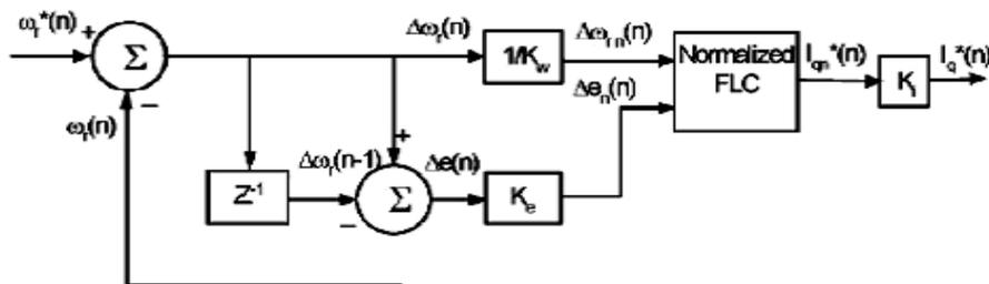
Fig.8. Fuzzy speed controller Construction
