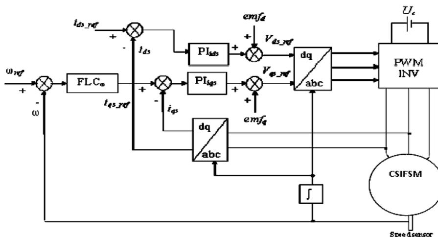
Fig.7. System Configuration of Field-Oriented CSI fed Synchronous Motor (CSIFSM) Control.
