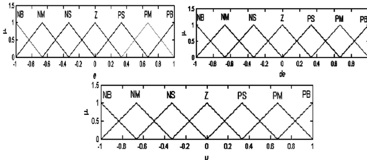
Fig.6. Membership functions for input  $e$ ,  $de$  and  $u$
