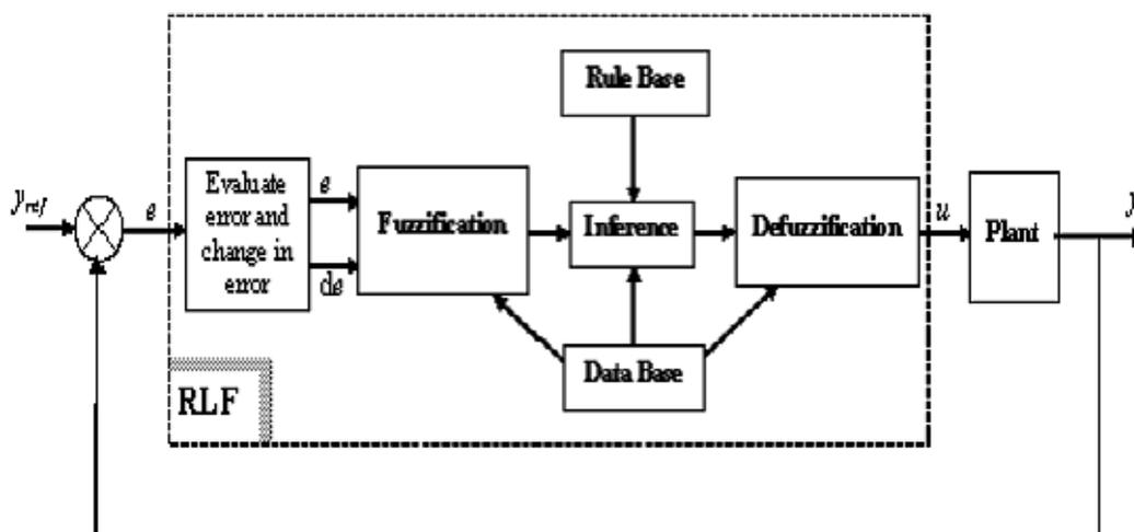
Fig.5 Basic structure of fuzzy control system
