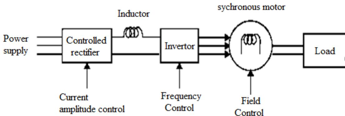
Fig.1 Drive configuration for open-loop CSI fed Synchronous Motor (CSIFSM) control
