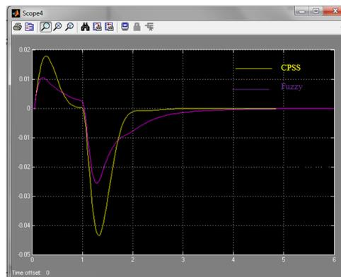
**Figure 10:** Rotor speed deviation for 5% change in mechanical power input with CPSS and Fuzzy PSS.
