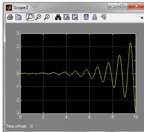
**Figure 9:** Rotor speed deviation for 5% change in mechanical power input with AVR and K5 Negative.
