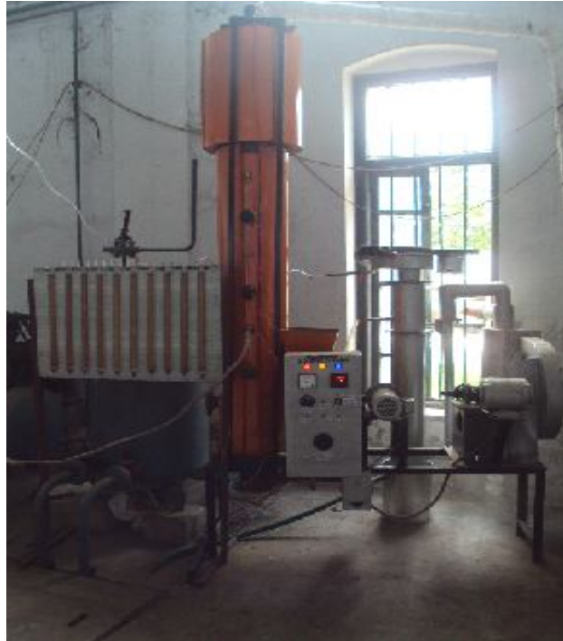
Fig. 1: Experimental fluidized bed gasification system
