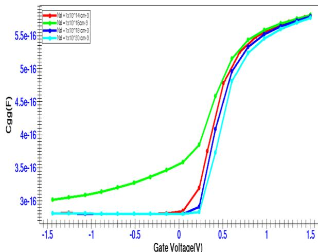
Fig.5. Gate capacitance for 1 nm gate length with 1nm oxide thickness
