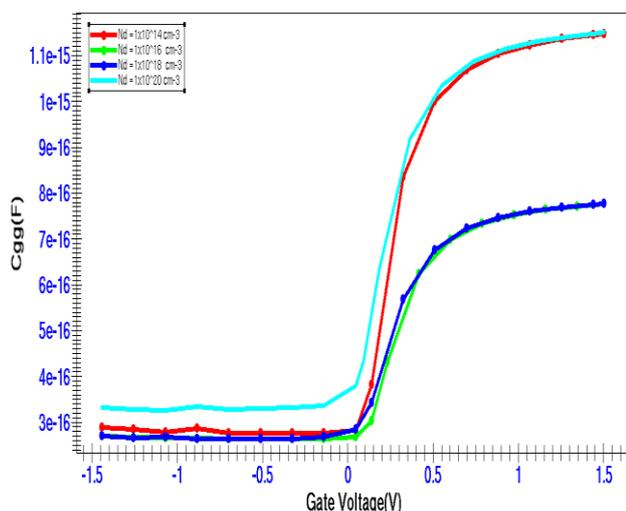
Fig.4. Gate capacitance for Gate length (Lg) of 5-nm with gate oxide thickness of 1-nm double gate T-shaped JLT.
