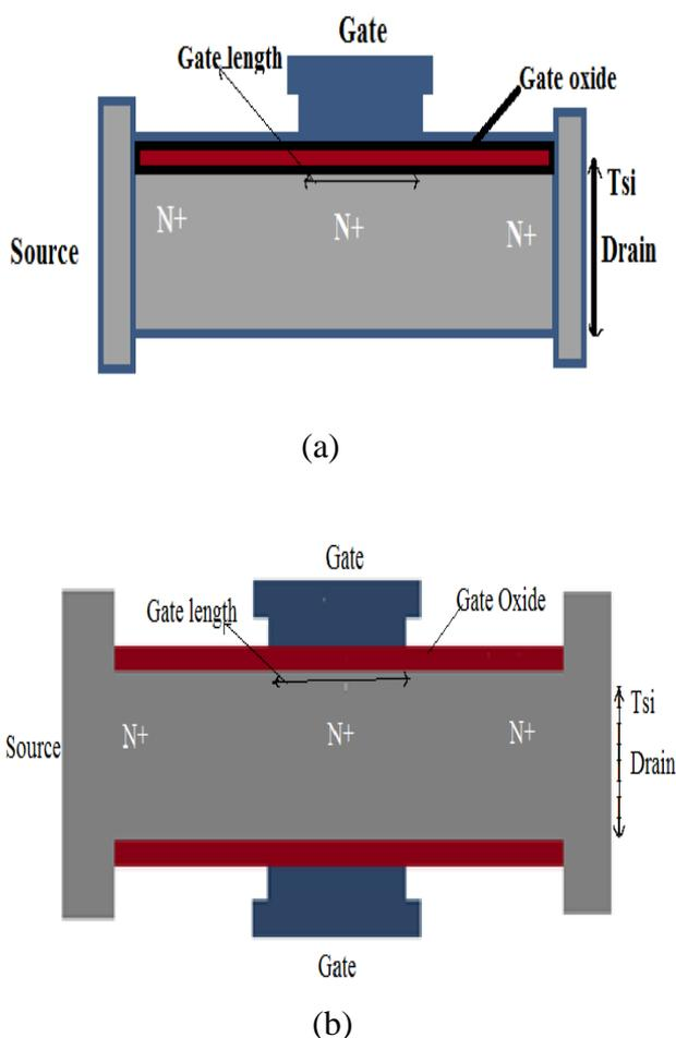
Fig.1. (a): 2D single gate; (b): double gate junctionless transistor.
