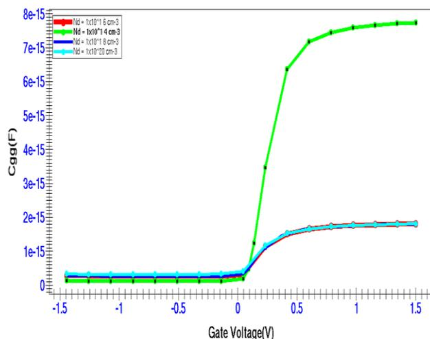
Fig.3. Gate capacitance for 19 nm gate length with 1nm oxide thickness
