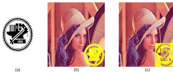
Fig.(3). Illustration of pixels in a watermark. (a) A monochrome watermark. (b) Area of p (yellow pixels). (c) Area of p' (yellow pixels).
