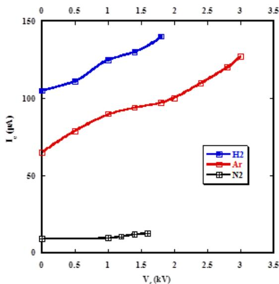
Figure 10: Influence of the focusing voltage applied to the focusing electrode on the electron current with different gases at discharge current of 0.4 mA and gas pressure of  $2 \times 10^{-3}$  mbar.
