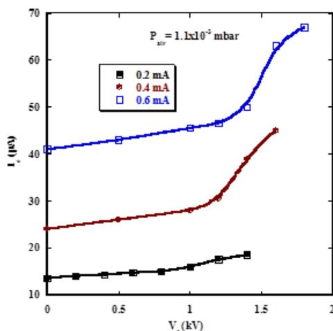
Figure 9: Relation between the focusing voltage applied to the focusing electrode and electron beam current with different discharge current at air gas pressure  $P= 1.1 \times 10^{-3}$  mbar.
