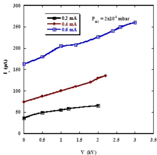
Figure 7: Relation between the focusing voltage applied to the focusing electrode and electron beam current with different discharge current at hydrogen gas pressure  $P= 2 \times 10^{-3}$  mbar.
