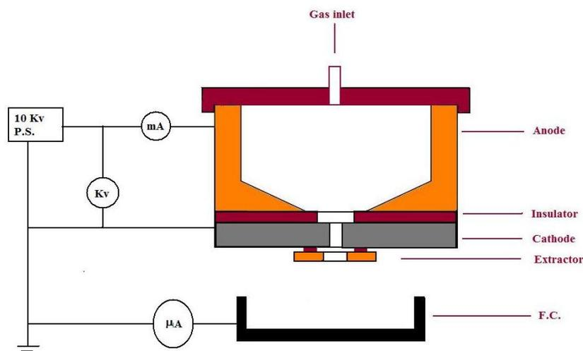
Figure 1: Schematic diagram of the electron source and its associated electrical circuit.
