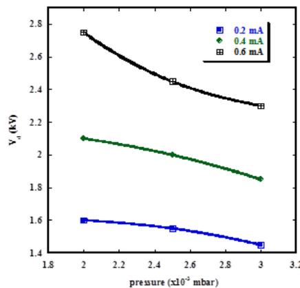
Figure 3: The discharge voltage as a function of gas pressure at different discharge currents.
