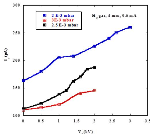
Figure 4: Relation between the focusing voltage applied to the focusing electrode and the electron beam current at different hydrogen gas pressures.
