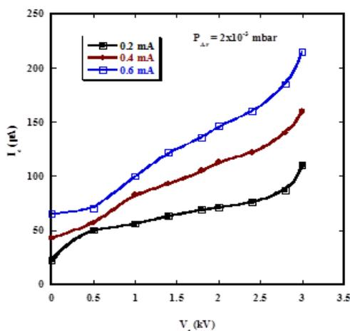
Figure 8: Relation between the focusing voltage applied to the focusing electrode and electron beam current with different discharge current at argon gas pressure  $P= 2 \times 10^{-3}$  mbar.
