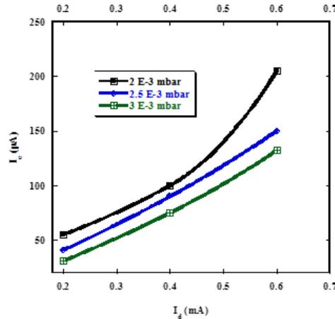
Figure 2: Relation between the discharge current and the electron beam current at different hydrogen gas pressures.
