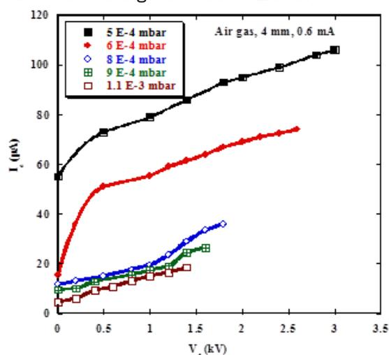
Figure 6: Relation between the focusing voltage applied to the focusing electrode and the electron beam current at different air gas pressures.
