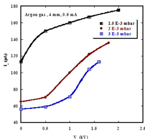
Figure 5: Relation between the focusing voltage applied to the focusing electrode and the electron beam current at different argon gas pressures.
