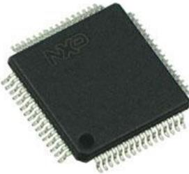
The microprocessor that has been used for this project is a 32 bit ARM7, CPU with real-Time emulation and embedded trace support that combines the microcontroller with 512 Kb of embedded high speed Flash memory. It has two 8 channel ADC ,single 10 bit DAC, two 32 bit timer/counter ,multiple serial interfaces including two UART ,two fast I2C, Capture, compare and PWM module.
