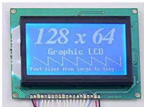
The **Graphical LCDs** are used to display customized characters and images. The Graphical LCDs used in many applications; they are used in video games, mobile phones, lifts etc. as display units. This LCD has a display format of **128x64 dots** and has yellow-green colour backlight. Here it is used to display all details of soldier such as speed, distance height and also their health parameter's
