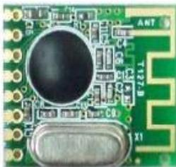
This is an FSK transceiver module, which is designed using Chipcon IC(cc2500).it is true single-chip transceiver, it is based on 3 wire digital serial interface and an entire phase-locked loop for precise local oscillator generation .it can be used in 2400-2483.5GHz ISM/SRD band system. it is high performance and low cost module.
