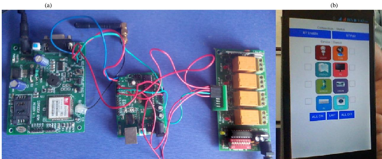
Figure 6: Real Implementation of GHAS (a) Real Prototype and (b) GHAS App Screen Shot
