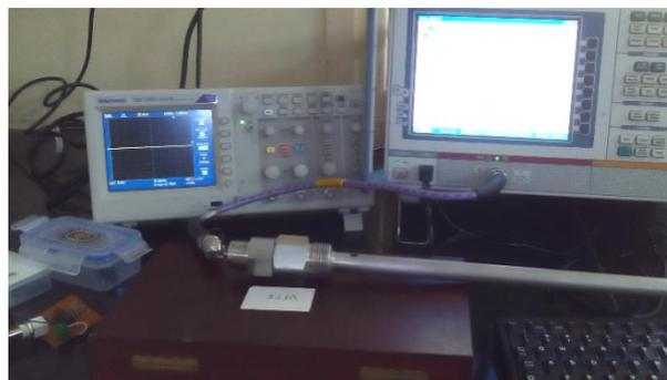
Fig 2. 2m Stainless steel waveguide testing with characteristic impedance of 50 Ω in air.
