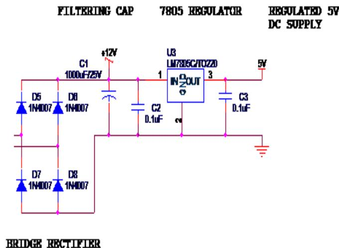
Figure 5: Power Supply design
