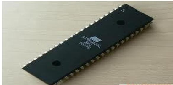
Figure 4: AVR ATmega32 Microcontroller
