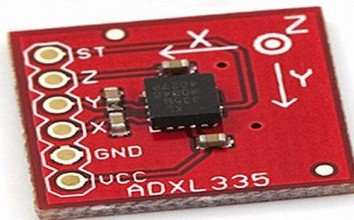
Figure 2: Accelerometer ADXL335
