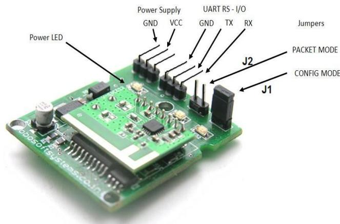
Figure 3: RF Trans-Receiver Module
