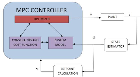
Fig.1 Basic Structure of MPC
