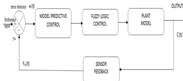
Fig.3 proposed controller design for temperature process
