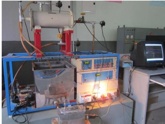
Fig.4 Experimental setup for temperature control process station
