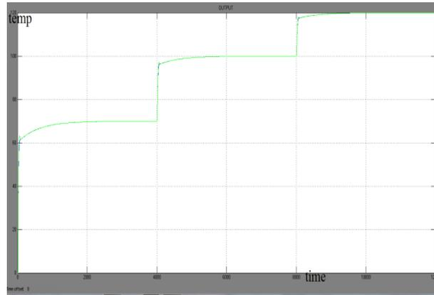
Fig.8 Response curve of MPC based Fuzzy controller action
