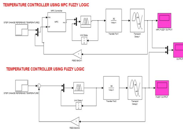
Fig.6 MATLAB simulation for proposed work
