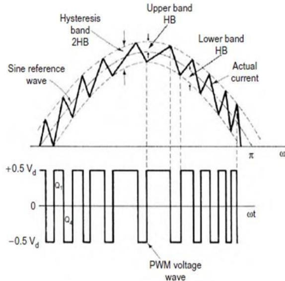
Fig. 5 Principle of hysteresis band current controller
