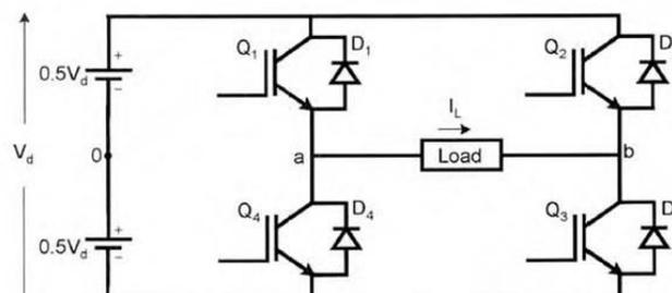
Fig. 1. Single Phase H bridge inverter
