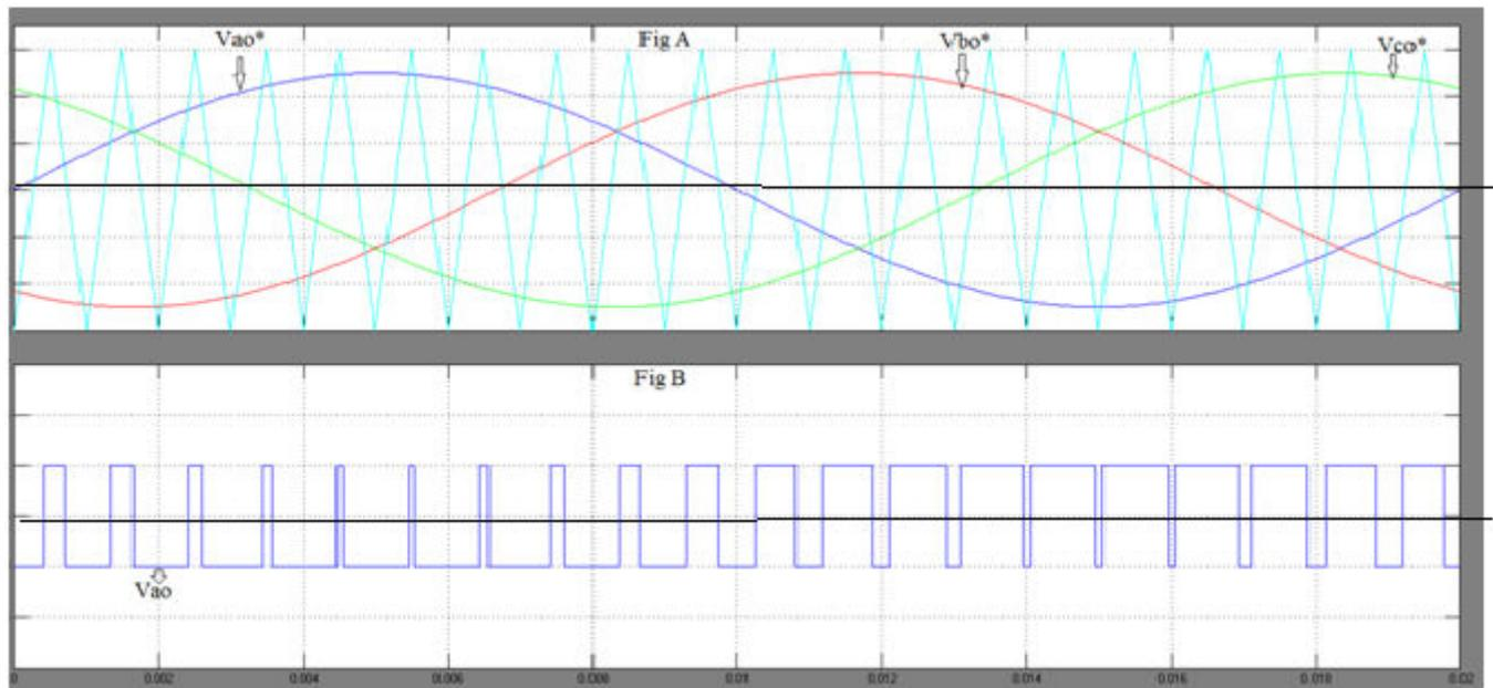
Fig. 4. Waveform of carrier wave and modulating wave and output voltage
