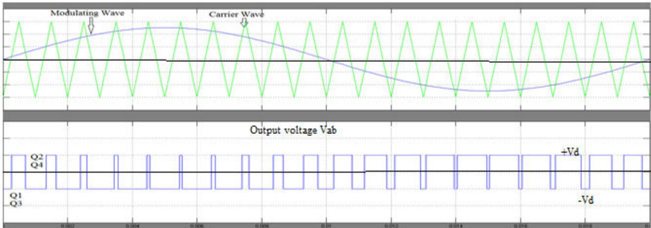
Fig. 2. Waveform of carrier wave and modulating wave
