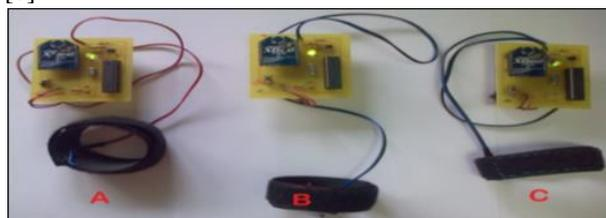
Figure 4: Heartbeat Monitoring Device using Zigbee [8].
