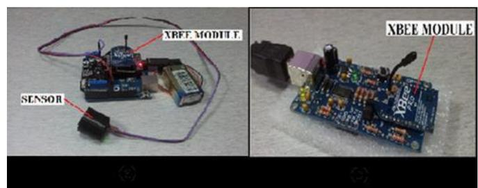
Figure 3: Preliminary Prototype Zigbee (Xbee) Transceiver.
