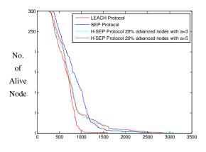
**Figure 4** Number of affive flowes per found in random deployment in square field (LEACH; SEP; H-SEP with m=0.2 and a=3; H-SEP with m=0.2 and a=5 for 2-level)
