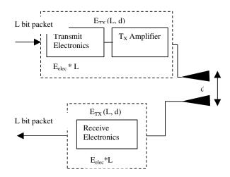
Figure 1 Radio Dissipation Model
