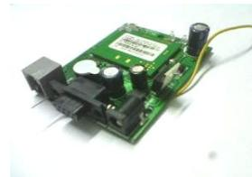
Fig. GSM modem
