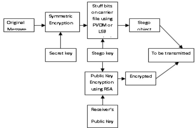
Figure 1: Proposed system – Sender’s side
