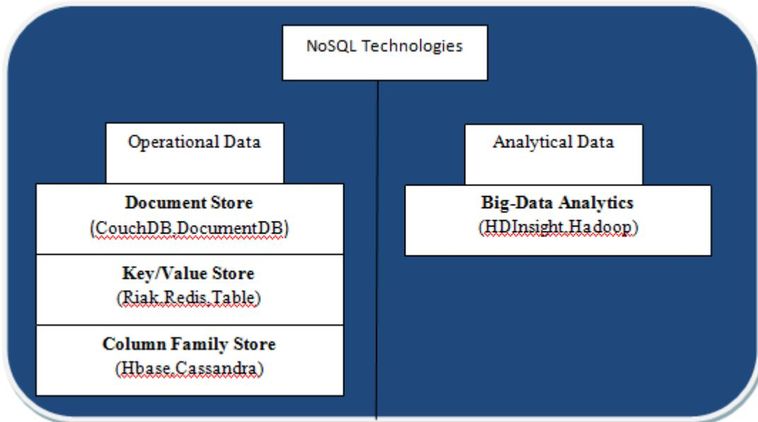
Figure 1: Azure data technologies categorized into two groups for NoSQL[2].
