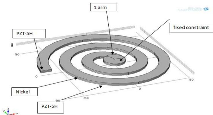
Fig.2: 1 arm spiral shaped bimorph piezoelectric transducer.
