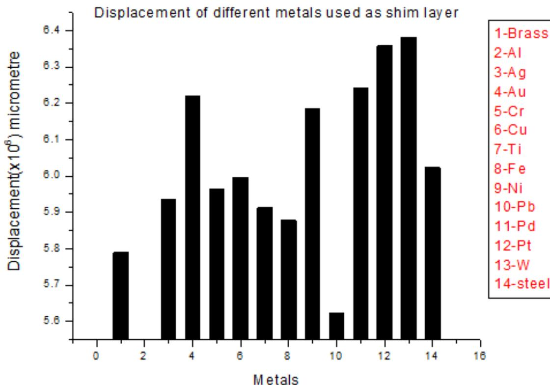
Fig.7: Graph to show the displacement of various metals used as shim layer.
