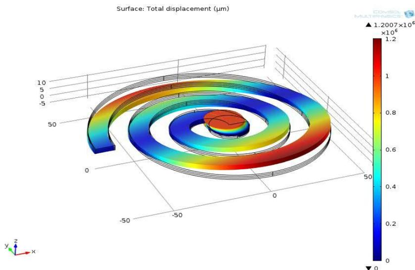
Fig.5: 1 arm spiral shaped PZT
