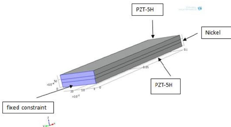
Fig.1: Rectangular shaped bimorph piezoelectric transducer.
