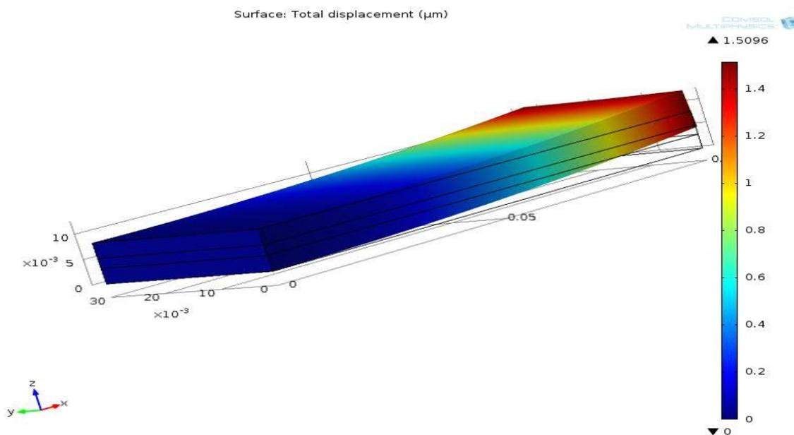
Fig.4: Displacement of rectangular bimorph PZT
