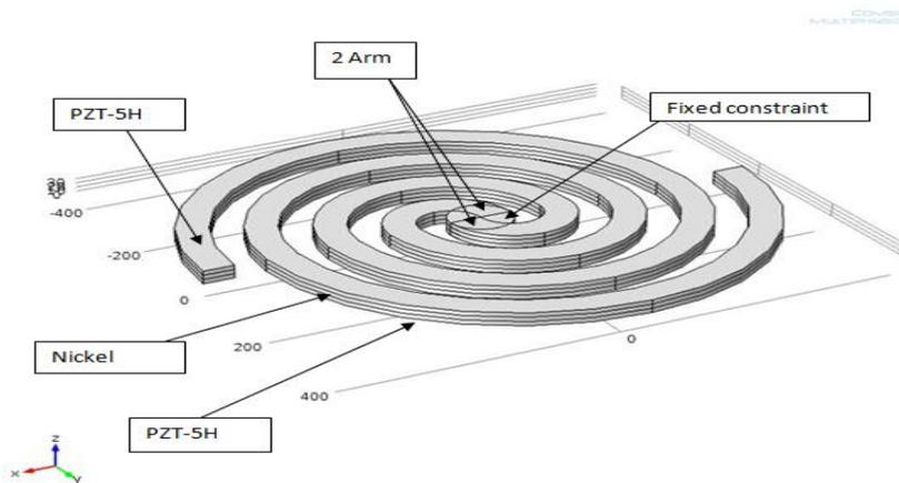
Fig.3: 2 arm spiral shaped bimorph piezoelectric transducer.
