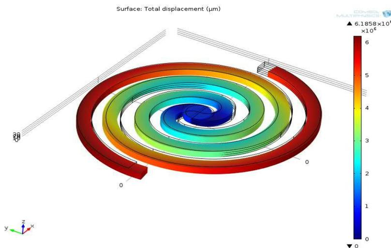
Fig.6: 2 arm spiral shaped PZT
