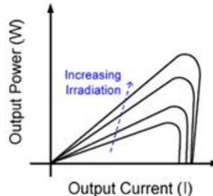
Figure 9: PV cell power characteristics
