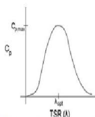
Figure 8 Power Coefficient Curve for a typical wind turbine
