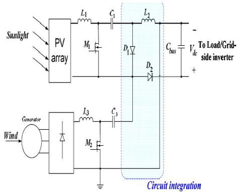
Figure 3: Proposed rectifier stage for a Hybrid wind/PV system
