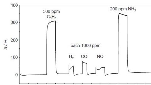
Fig.6. Sensitivity  $S$  over  $t$  at 3 Hz and 350 °C.
