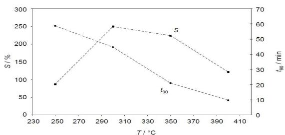
Fig.4 Sensitivity (left axis) and sensor response time (right axis) at a fixed frequency of 3 Hz.
