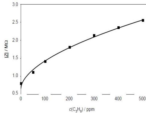
Fig.5. Sensor impedance  $|Z|$  at 3 Hz over the C<sub>3</sub>H<sub>8</sub> concentration at 350 °C.
