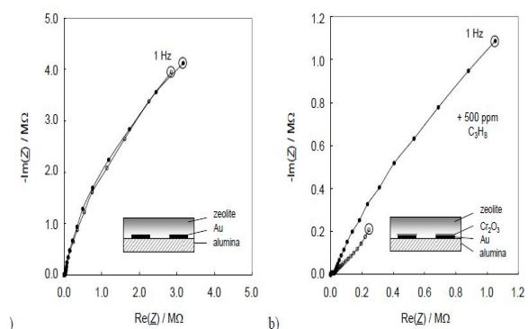
Fig.1. Line graph shown a gas and 500 ppm C<sub>3</sub>H<sub>8</sub> added to the base gas of 2.5 % H<sub>2</sub>O and 10 % O<sub>2</sub> in N<sub>2</sub>. T = 300 °C.
