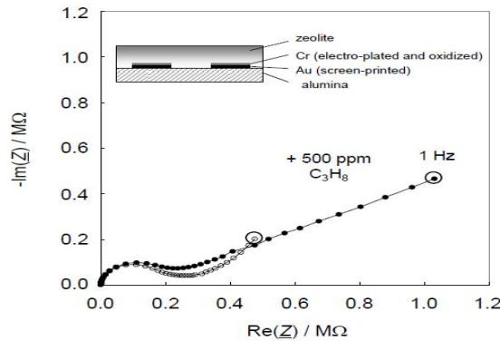
Fig.3 Graph of a thick film sensor with and without 500 ppm C<sub>3</sub>H<sub>8</sub> at 350 °C
