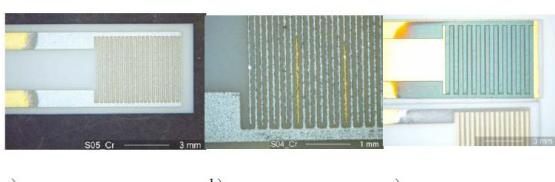
Fig.2. Micro view of the sensor during the chromium electroplating and oxidation Process.
