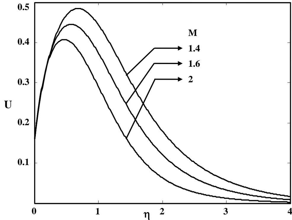
Fig.3 Velocity profiles for different M
