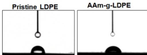
**Figure 3a:** Optical photographs of water droplets taken during contact angle measurement on the smooth (pristine LDPE) and rough (AAM-g-LDPE) surface.
