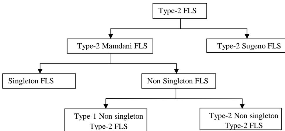
Fig.3. Classification of Type-2 Fuzzy logic system
