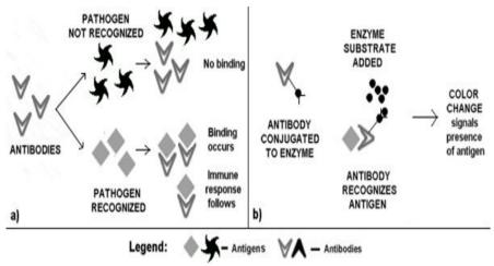
Fig. 3: Systematic diagram of Antibody-Antigen Interaction (Source: [1])
