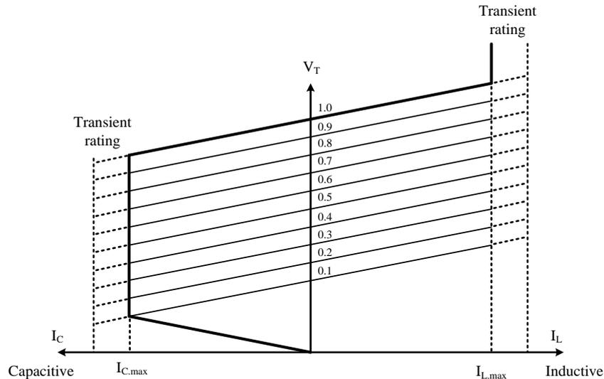
Fig. 2 V-I Characteristics of STATCOM
