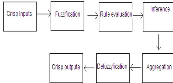
Figure 1. Fuzzy logic controller block diagram
