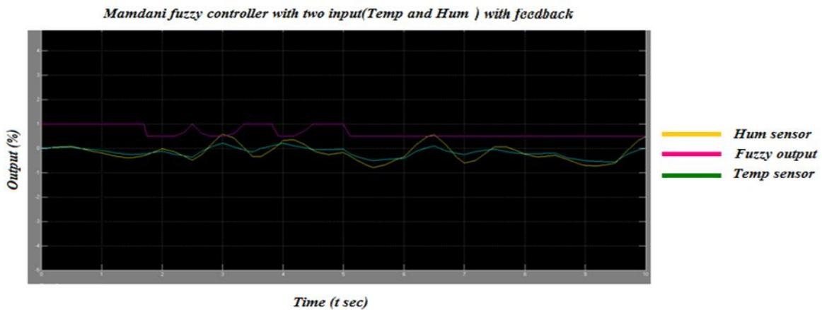
Figure 4. Mamdani Fuzzy controller with feedback signal
