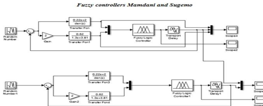
Figure 2 Two fuzzy controllers with two inputs temp and humidity
