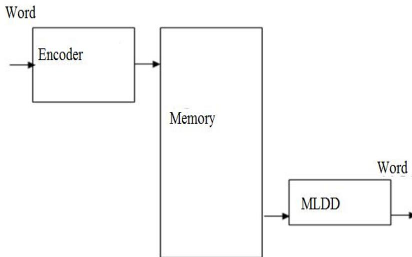
Fig. 2 Memory system schematic with MLDD
