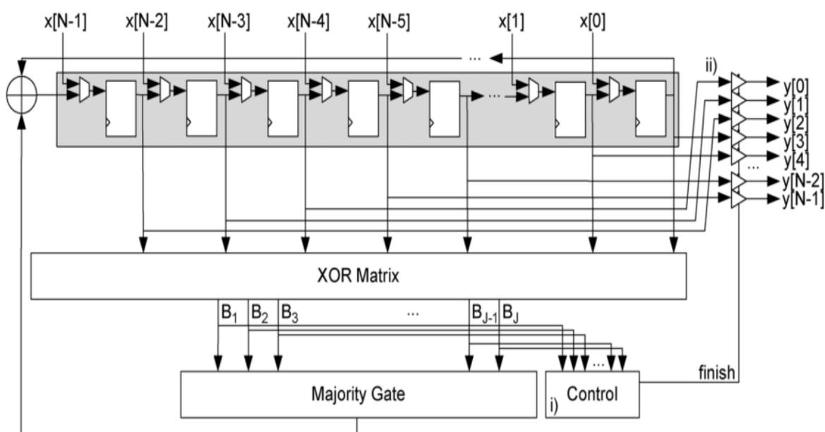
Fig. 3 Schematic Of The Proposed MLDD With Control Logic
