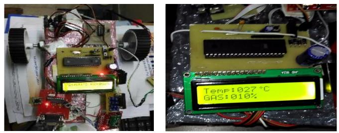
Figure 4: Final implementation of Air pollution monitoring Swarm robots.
