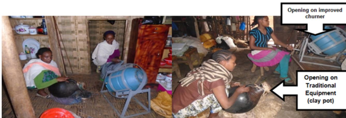
Figure 1. Simultaneous churning by Improved and traditional churner (clay pot).
