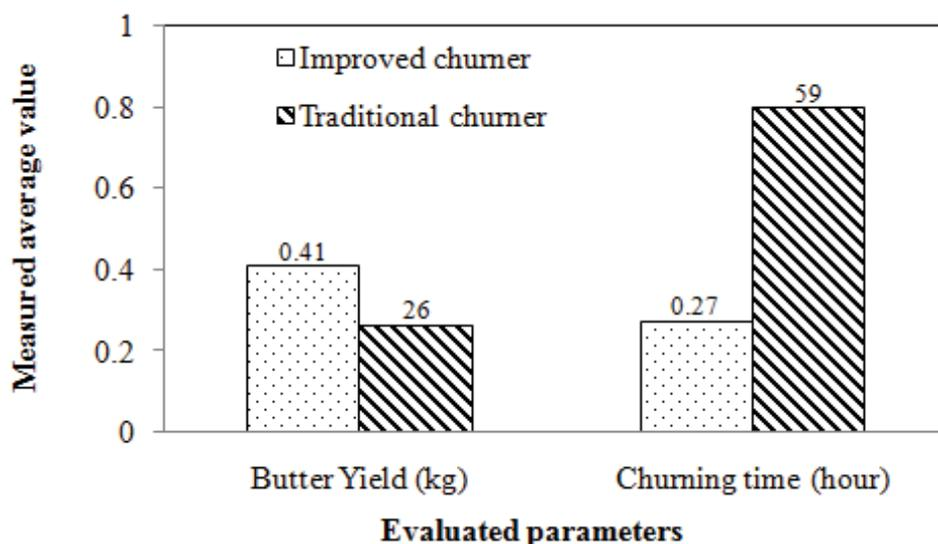
**Figure 4.** Butter making efficiency of improved and traditional (clay pot) churning equipments.
