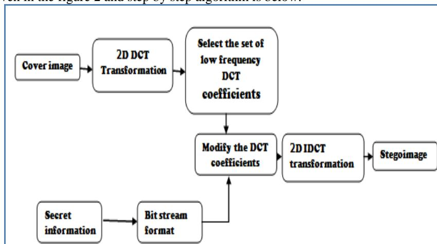
Figure 2 Block diagram of DCT Image Steganography
