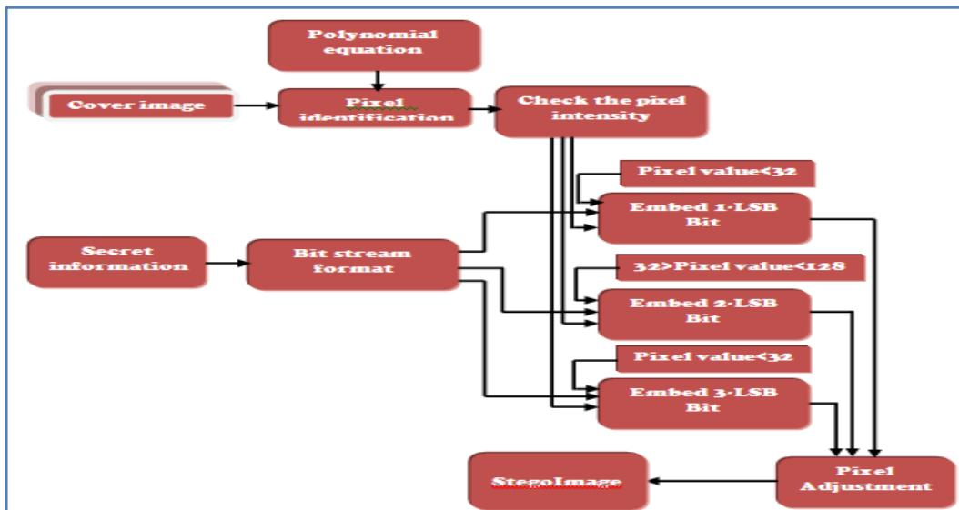
Figure 3 Block diagram of POLPA image steganography
