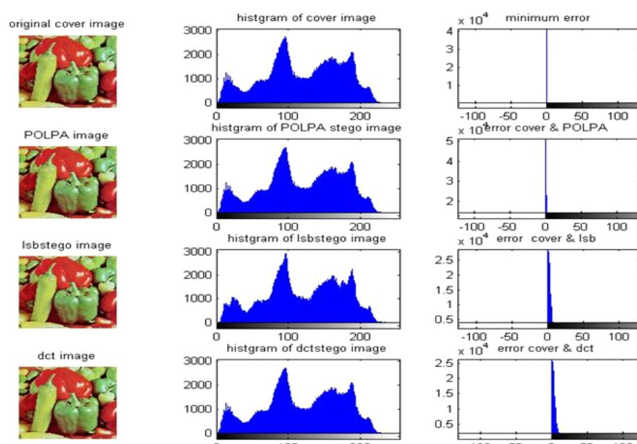
Figure 6 Histogram analyses for LSB DCT &POLPA on JPEG format
