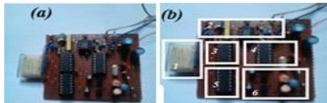
**Figure 1: Complete fluxgate sensor system.**
