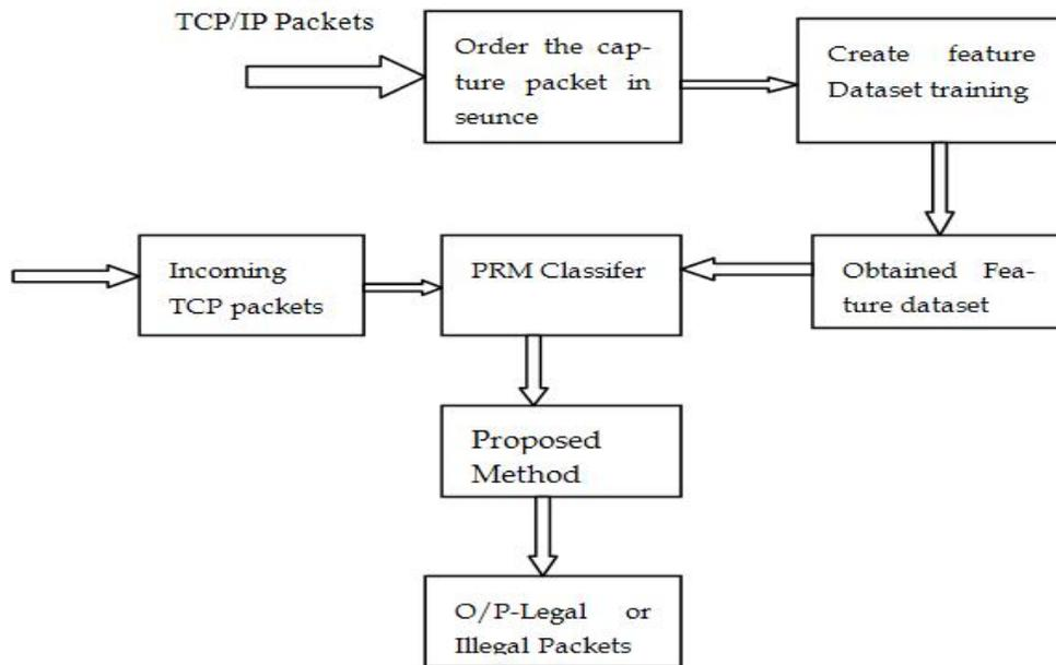
**Fig .Block Diagram for covert channel detection**
