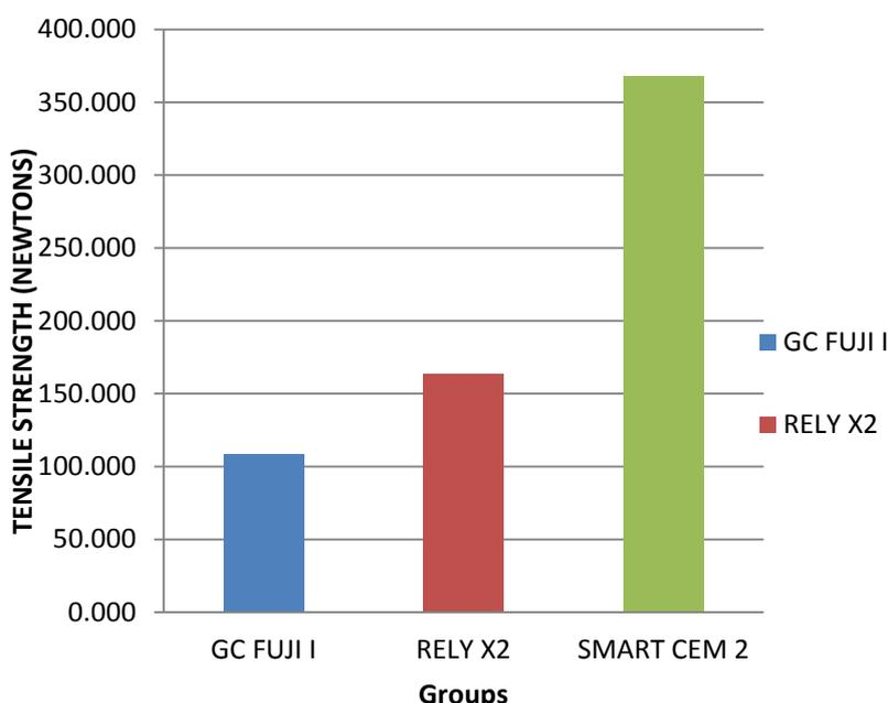
**Graph 1.** Mean tensile bond strength of the cements.
