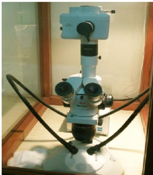
**Figure 1.** LEICA WILD M 3 Z stereomicroscope.
