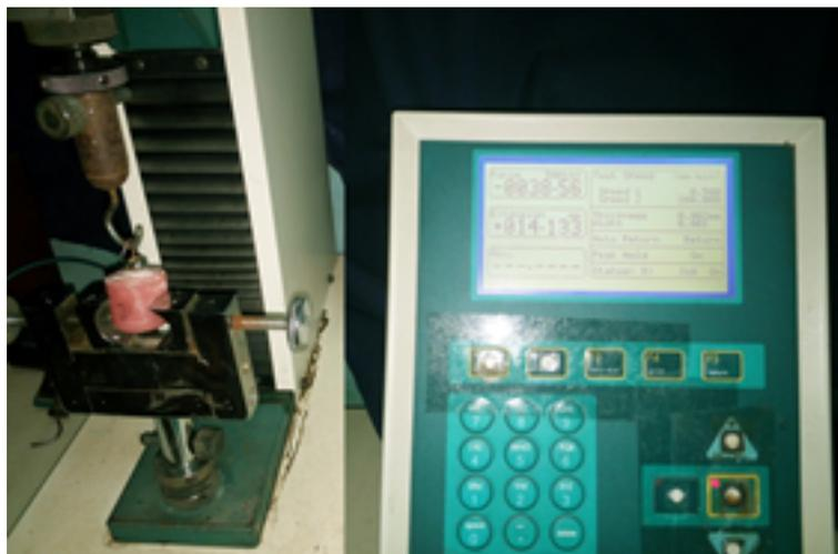
Figure 4. Teeth tested using Instron testing machine to measure tensile bond strength.
